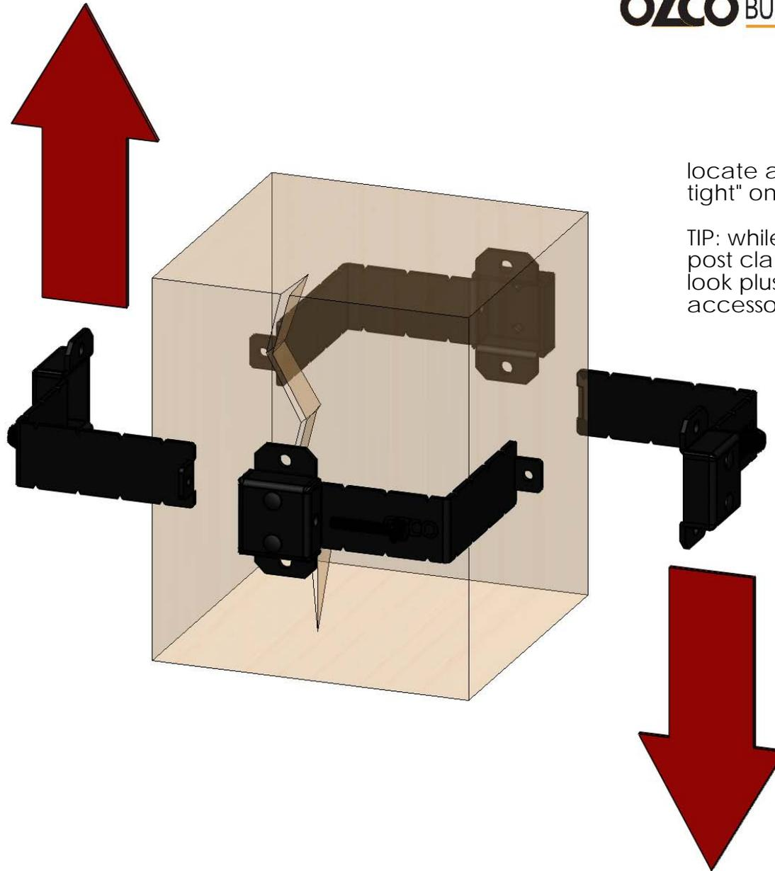
locate and install post band "finger tight" on post in desired location.
