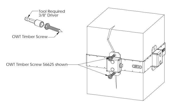
when additional strength is required, install OWT Timber Screws (sold separately)
