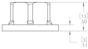
When using 1/2" OWT-Timberbolts, drill out this hole to  $\emptyset$ 5/16"
