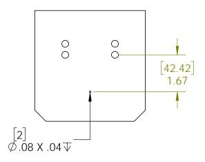
Material: ASTM A36 Steel Finish: Black Powder Coat
