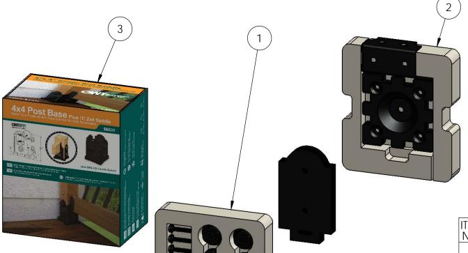
PART NUMBER ITEM QTY. **DESCRIPTION** NO. Insert, Insert, Rail Rail Saddle Saddle Insert, Insert, Rail Rail Saddle Saddle Box, 3 Box, 56630 56631
