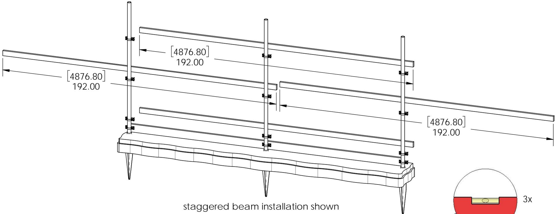
staggered beam installation shown
