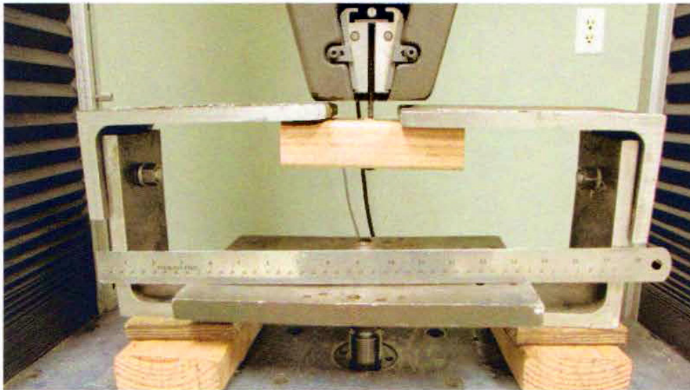
Figure 3: Screw pull through test setup
