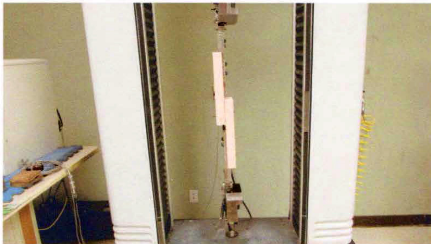
Figure 6: Lateral load test setup for screw
