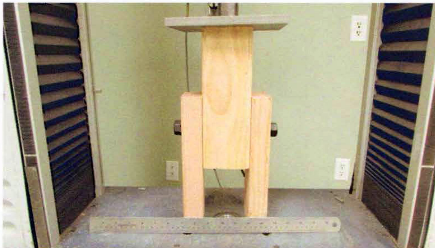
Figure 8: Lateral load test setup
